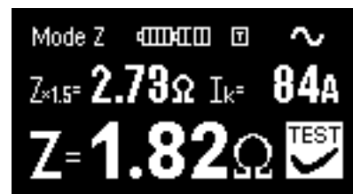
Fig. 3.8b Loop measurement result (Detailed display mode, example)
