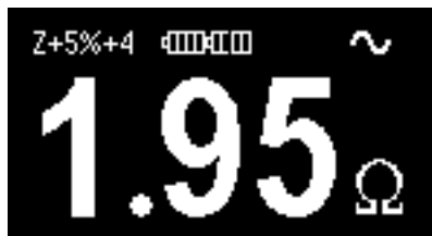
Fig. 3.11 Example of Loop/Line resistance result which takes into account the measurement error
