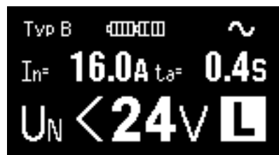
Fig. 3.17b Phase voltage present on the test tip (Detailed display mode)
