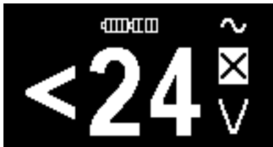
Fig. 3.1a Voltage < 24\text{ V} (Basic display mode, example)
