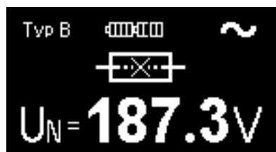
Fig. 3.2 The symbol of blown fuse (Detailed display mode, example)
