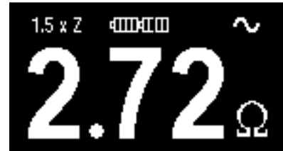
Fig. 3.10 Example of Loop/Line resistance multiplied by a factor 1.5
