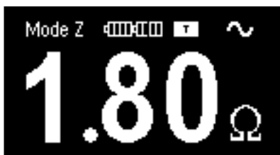
Fig. 3.8a Loop measurement result (Basic display mode, example)
