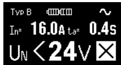
Fig. 3.1b Voltage < 24\text{ V} (Detailed display mode, example)
