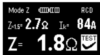
Fig. 3.15b Loop measurement result, RCD (Detailed display mode, example)
