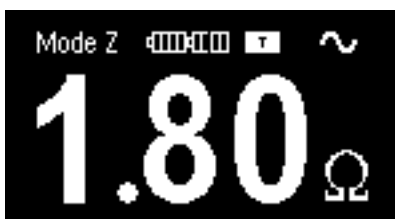
Fig. 3.5a Indication of high temp. (Basic display mode, example)
