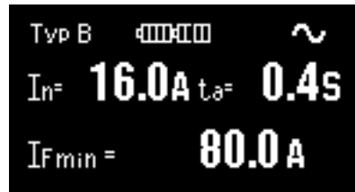
Fig. 3.16. Example of fuse parameters and minimal required fault current
