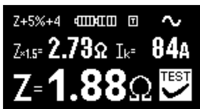
Fig. 3.13 Example of Loop/Line resistance result which takes into account the measurement error
