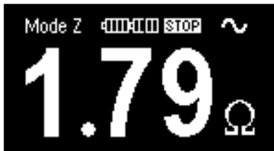
Fig. 3.6a Max. temp. exceeded (the STOP icon)
