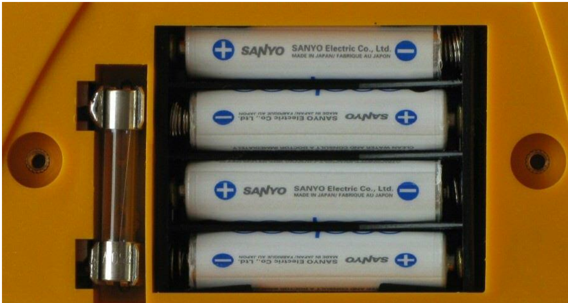
Fig. 4.1 Correct batteries/accumulators polarity and the fuse location
