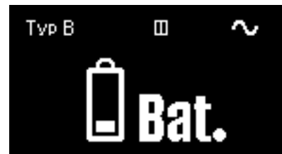
Fig. 3.4b Low battery after the START key was pressed
