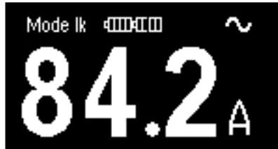
Fig. 3.9 Example of prospective fault/short-circuit current
