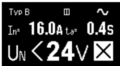
Fig. 3.4a Indication of low battery (Detailed display mode, example)
