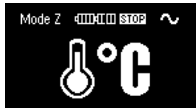
Fig. 3.6b Max. temp. exceeded icon (after the START key is pressed)
