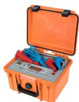
**LKN-1500 cable locator - transmitter**
